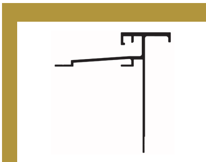
PLASTER PARAPET CAP
